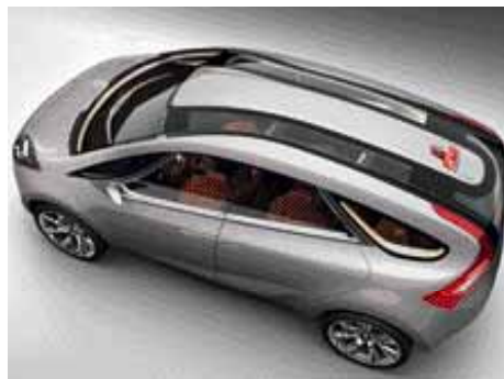
Exciting perspectives: The glazing components on the i-mode concept vehicle, from the windshield to the roof module to the rear window, are made of Makrolon®.
