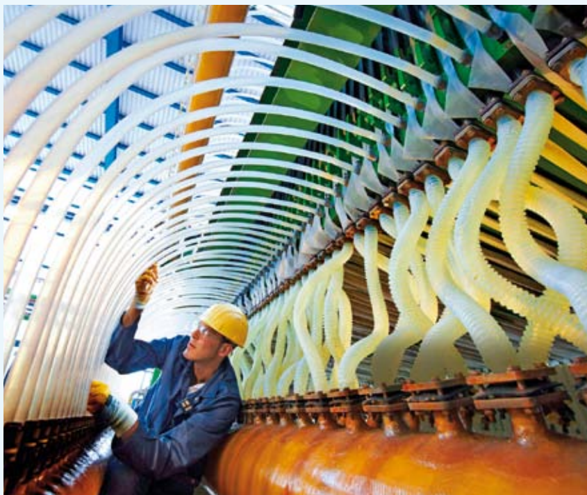
Plant assistant Jörg Bähler inspects inlet pipes on the oxygen depolarized cathode, co-developed by Bayer, which gives an energy saving of some 30 percent in the production of chlorine.
