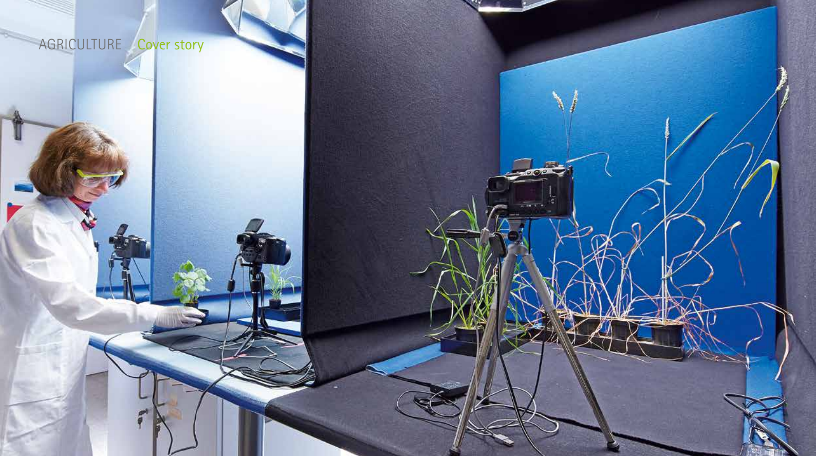
Cereal models: the wheat plants in the Crop Performance Lab will be photographed every six minutes over their entire lifespan. Petra Guer then turns the photos into time lapse films which allow the researchers to track how the plant morphology changes over time and in response to different active ingredients.
