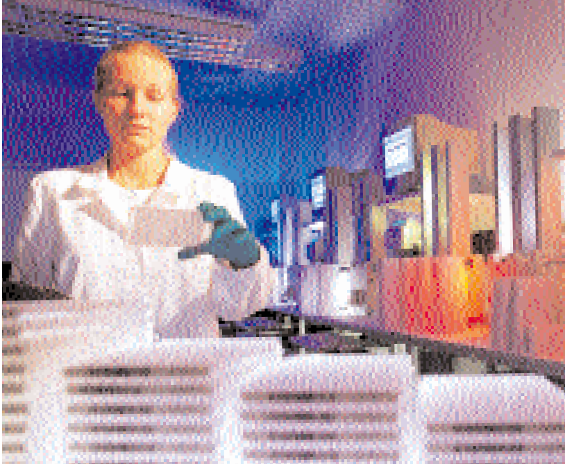
At the pharmaceutical research center in Wuppertal, Marina Breuhaus inspects and sorts microtiter trays. Once these trays have been filled with test substances, they are passed through a high-throughput screening machine for evaluation of substance efficacy.
