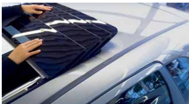
Innovation in automotive engineering: the Makrolon® sunroof
