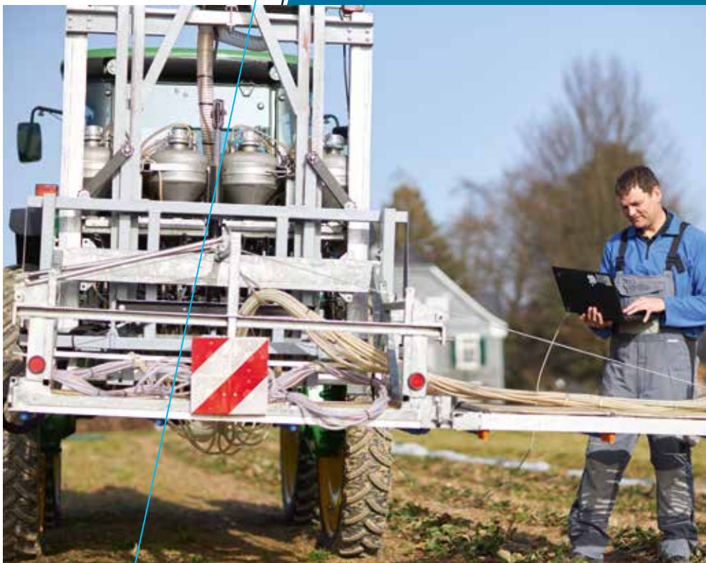
Spray tests at Bayer's in-house testing station Gut Höfchen.
