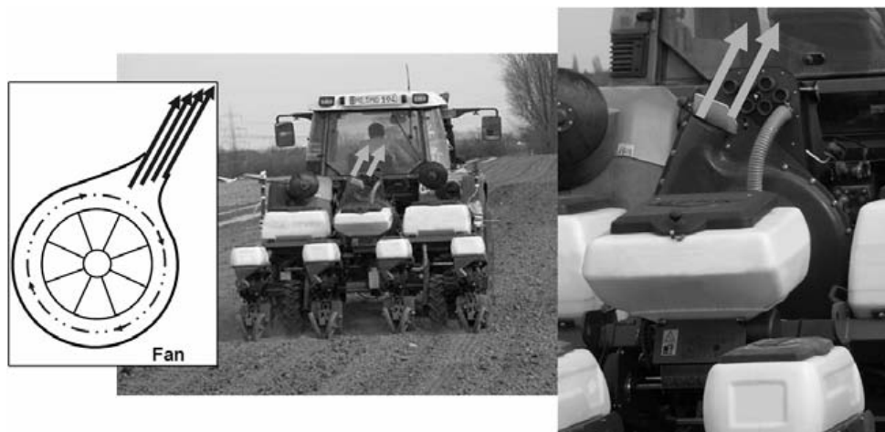
Figure 8 Standard vacuum-pneumatic drilling machine with an upward directed air-stream outlet, directly from the fan
