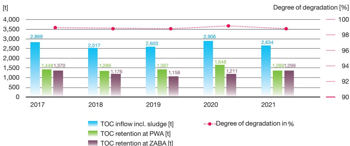
Fig. 12: TOC degradation at the process water and wastewater treatment plants [t = metric tons].
