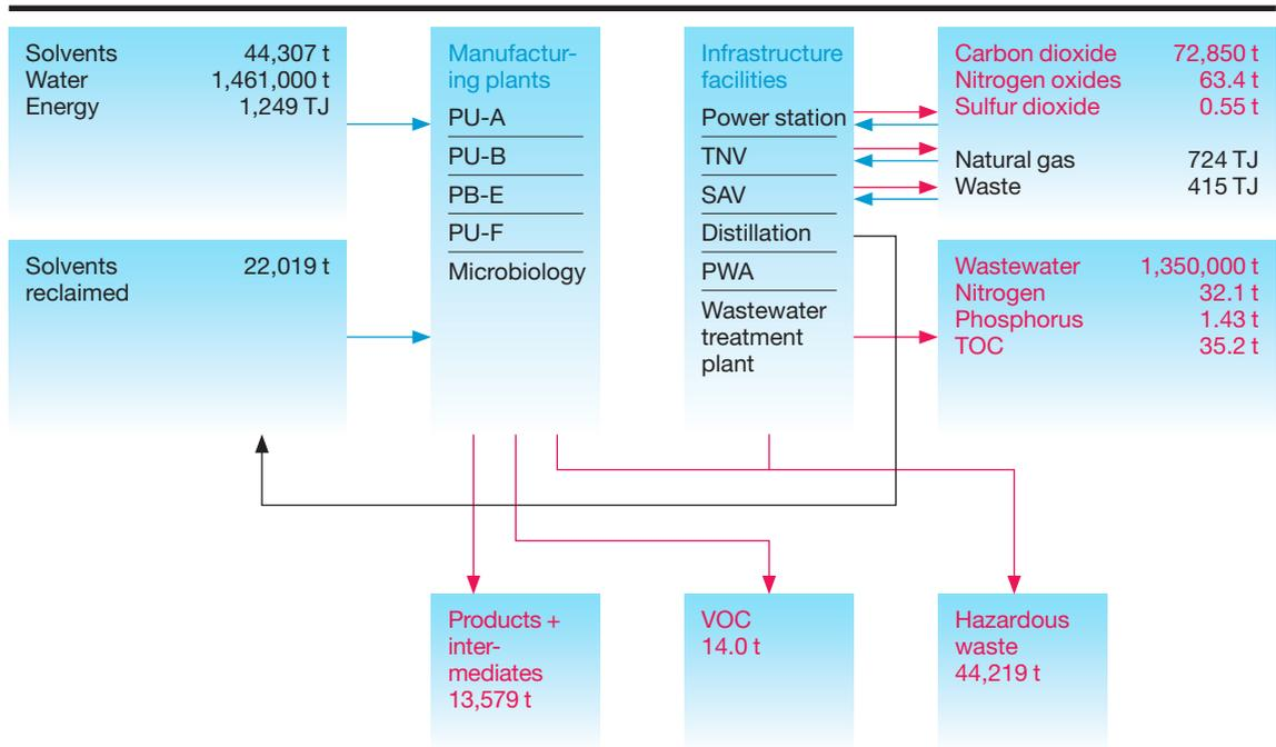
Fig. 6: Simplified overview of incoming and outgoing material flows in 2021 [t = metric tons; TNV = thermal afterburner; SAV = hazardous waste incinerator; PWA = process water treatment plant].
